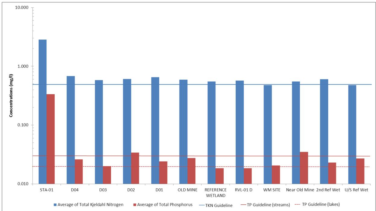
**Figure 2. Nutrient concentrations across monitored sites, mean values are shown for STA-01, OLD Mine, Reference Wetland, RVL-01D and WM site all other sites are based on single results value.**
