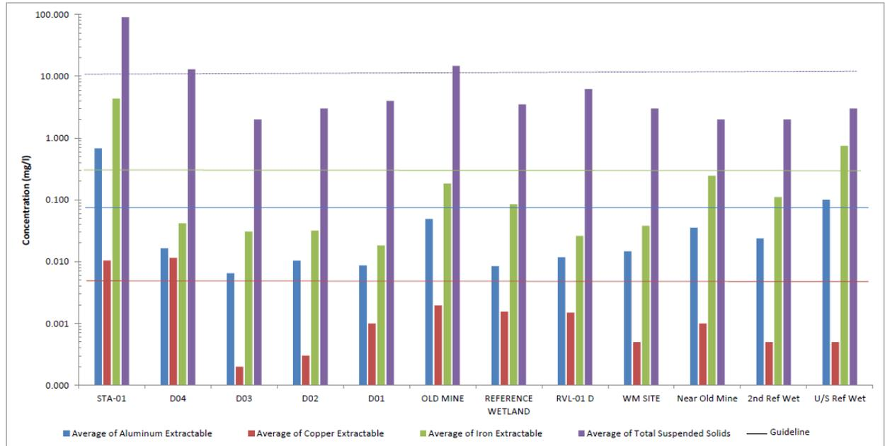
**Figure 3. Metal and TSS cocentrations across monitored sites, mean values are shown for STA-01, OLD Mine, Reference Wetland, RVL-01D and WM site all other sites are based on single results value.**
