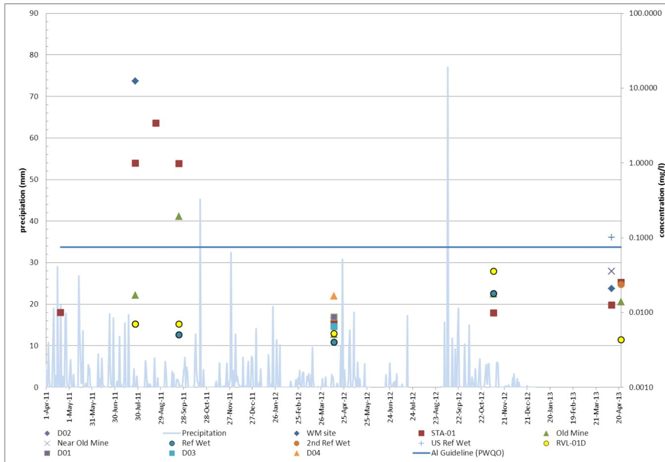
Figure 3. Precipitation and aluminum (Al) results for monitored sites.
