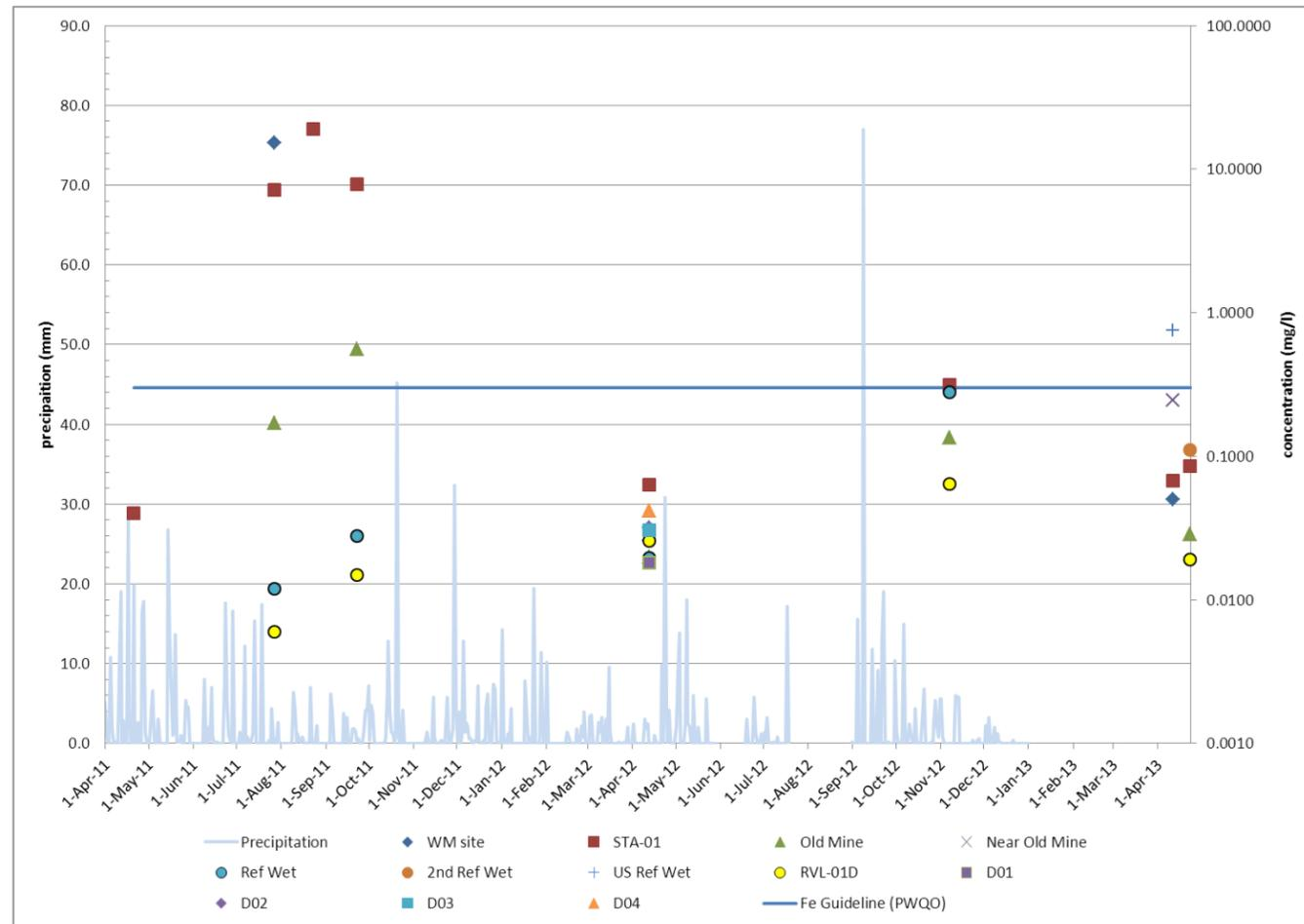
Figure 5. Precipitation and iron (Fe) results for monitored sites.
